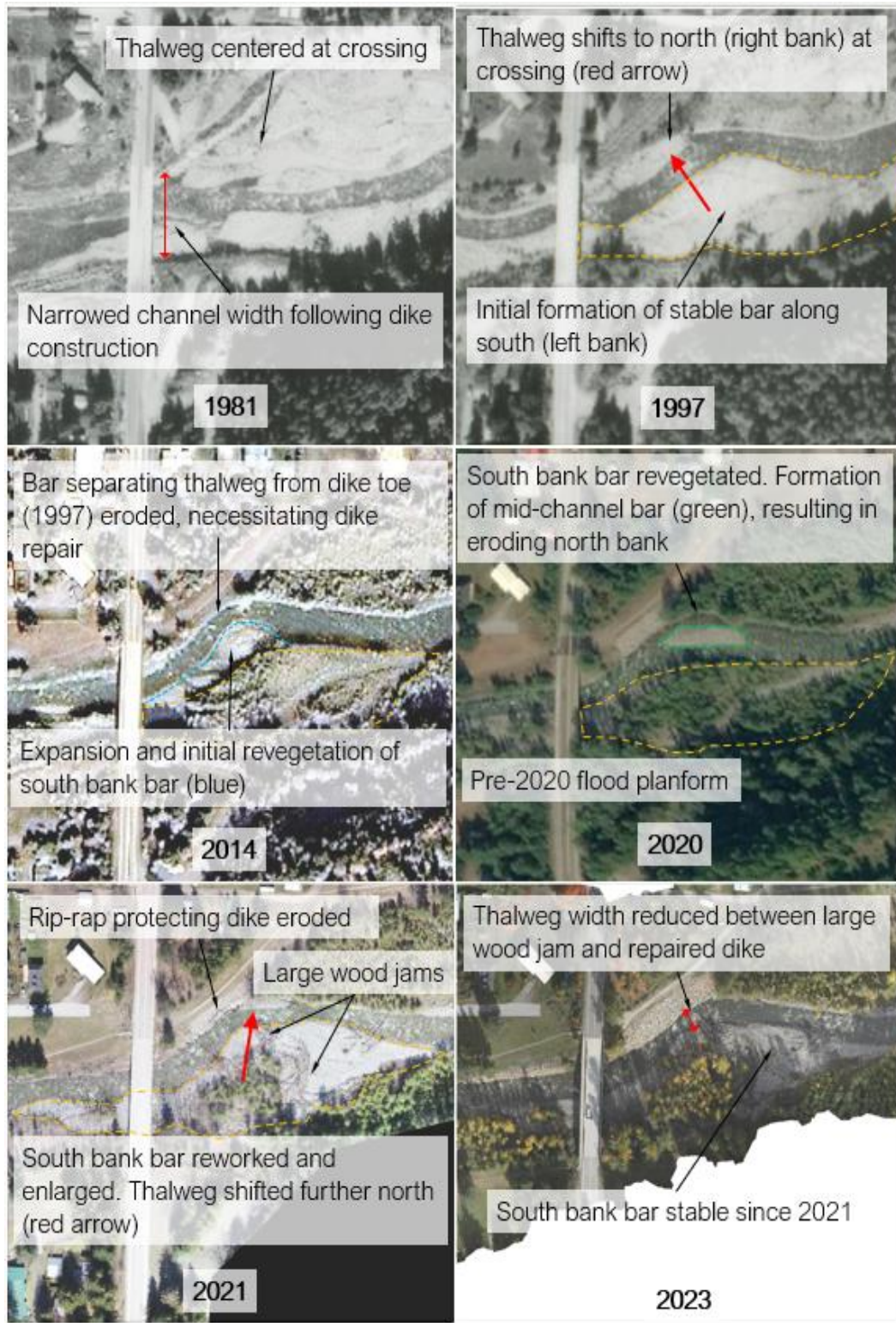
Figure 10: Comparison of historical imagery at the Bridge from 1981 (first available image following dike construction) to 2023. The channel thalweg has shifted northward to the dike, where it has remained in contact for approximately 40 years.
