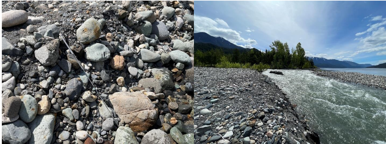
Photo 5: Overview of bed material (gravels and cobbles) at the edge of an active bar upstream of the Bridge (left; PC-2; note 60 cm steel folding rule for scale) and near the mouth of Carpenter Creek (right; PC-1). Note the slightly greater proportion of sand and pebbles nearer the mouth.
